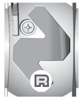
IMPORTANT! To avoid damaging the motors and gears, stop the vehicle before shifting from forward to reverse. Once your child is completely comfortable with operating the vehicle in the forward mode, introduce reverse.
